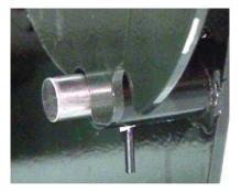
However, if you wish to utilize this "pin", it must be engaged immediately after you get the carpet started on the Roll-Up Side Cradle (approx. 3-5 turns). You will not be able to engage the "pin" once a larger/heavier piece has begun to be rolled up! In addition, once the "pin" is engaged, you will no longer be able to fold up the Roll-Up Cradle or use the Roll Dump Mechanism on this cradle.
