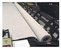
IMPORTANT NOTE: IF YOU CONTINUE THE ROLL-UP PROCEDURE BY PRESSING THE JOG BUTTON INSTEAD OF THE FOOT SWITCH TAPE, THE MACHINE WILL NOT STOP AUTOMATICALLY AT YOUR PRE-SET LENGTH. BE SURE TO USE THE FOOT SWITCH TAPE AFTER YOU HAVE GOT THE CARPET STARTED SO THIS FUNCTION CAN PERFORM PROPERLY.
