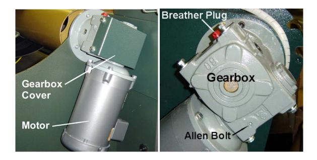
Use only 7 ounces of oil per gearbox, <u>do not totally fill gearbox</u>! Quaker State Synthetic Gear Oil is recommended but any brand 75W to 90W Synthetic Gear Oil or High Pressure Gear Oil is acceptable.
